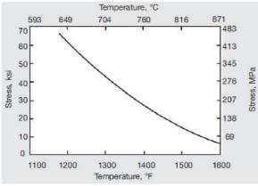
Figure 23 – 100-hr rupture strength of transverse specimens from joints alloy 625 made by gas-tungsten-arc process.
