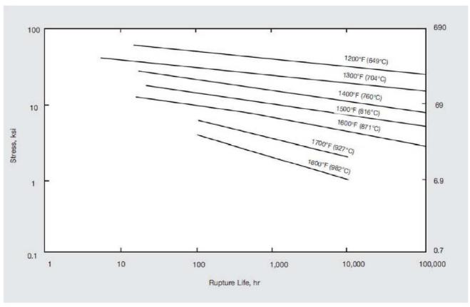
Figure 22 – Rupture strength of Welding Electrode 112 all-weld metal.
