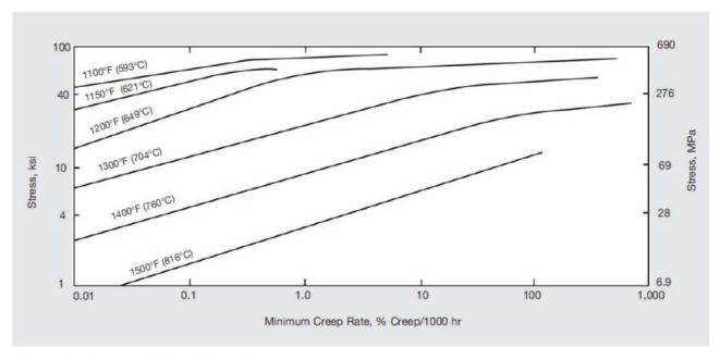
Figure 13 - Creep strength of annealed material.
