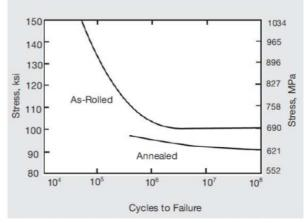
Figure 7 – Fatigue strength at room temperature of hot-rolled round (5/8-in. diameter).
