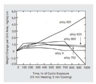
Figure 15 – Scaling resistance at 1800°F
