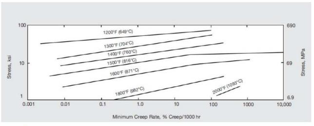
Figure 11 - Creep strength of solution-treated material.
