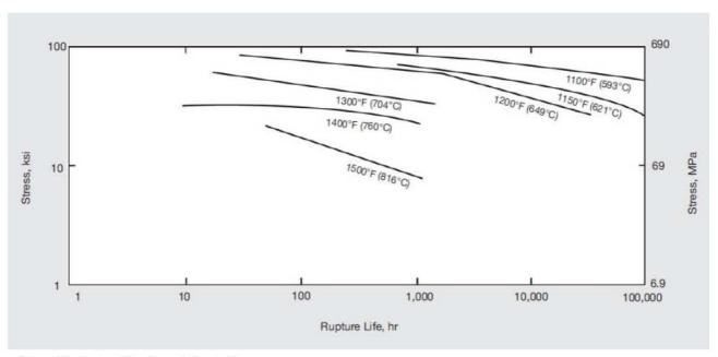
Figure 14 - Rupture life of annealed material.
