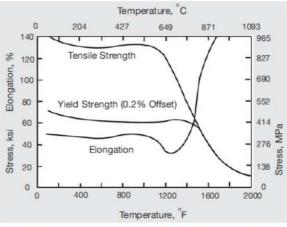
Figure 3 – High-temperature tensile properties of annealed bar.
