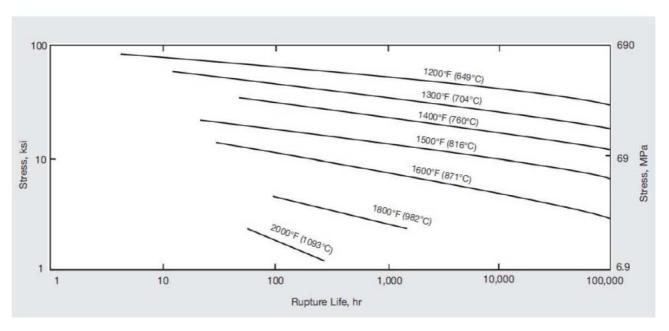
Figure 12 - Rupture life of solution-treated material.
