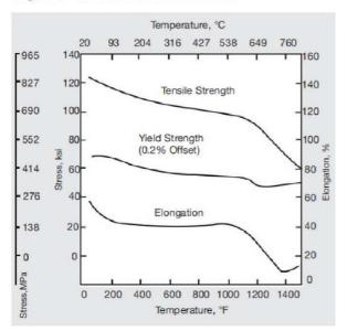
Figure 19 – High-temperature tensile properties of transverse alloy 625 welds
