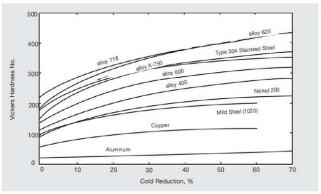
Figure 18 - Effect of cold work on hardness.
