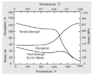
Figure 5 – High-temperature tensile properties of hot-rolled solution-treated rod.
