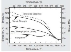
Figure 21 – High-temperature tensile properties of deposited weld metal from weld made in alloy 625
